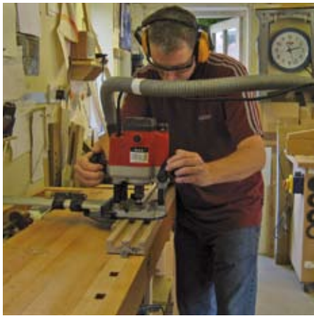
Routing the housings for the tubes
