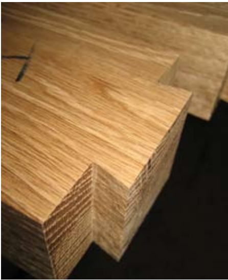
The rails with heavy-duty dovetails
