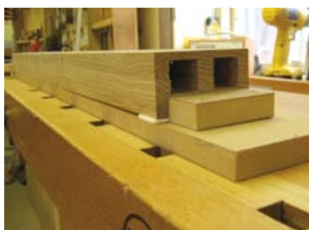
Jig with spacer to give taper
