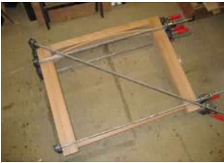
Gluing-up end assembly – note the spacer bar and diagonal clamp to maintain square
