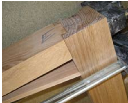
Gluing-up the side rails
