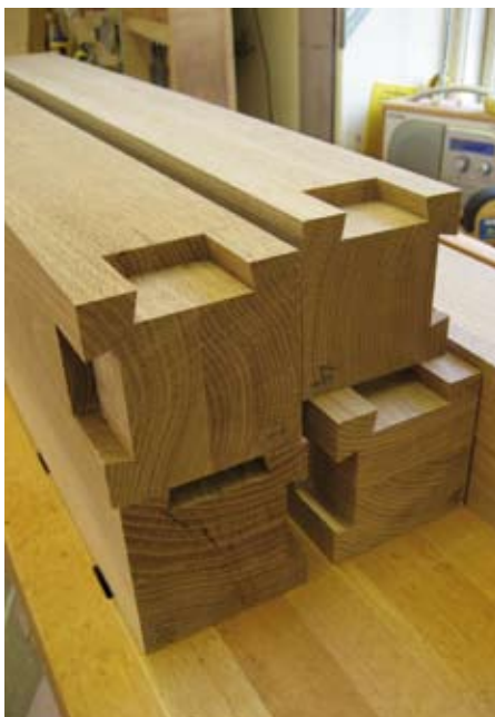
Glued up legs with dovetail sockets
